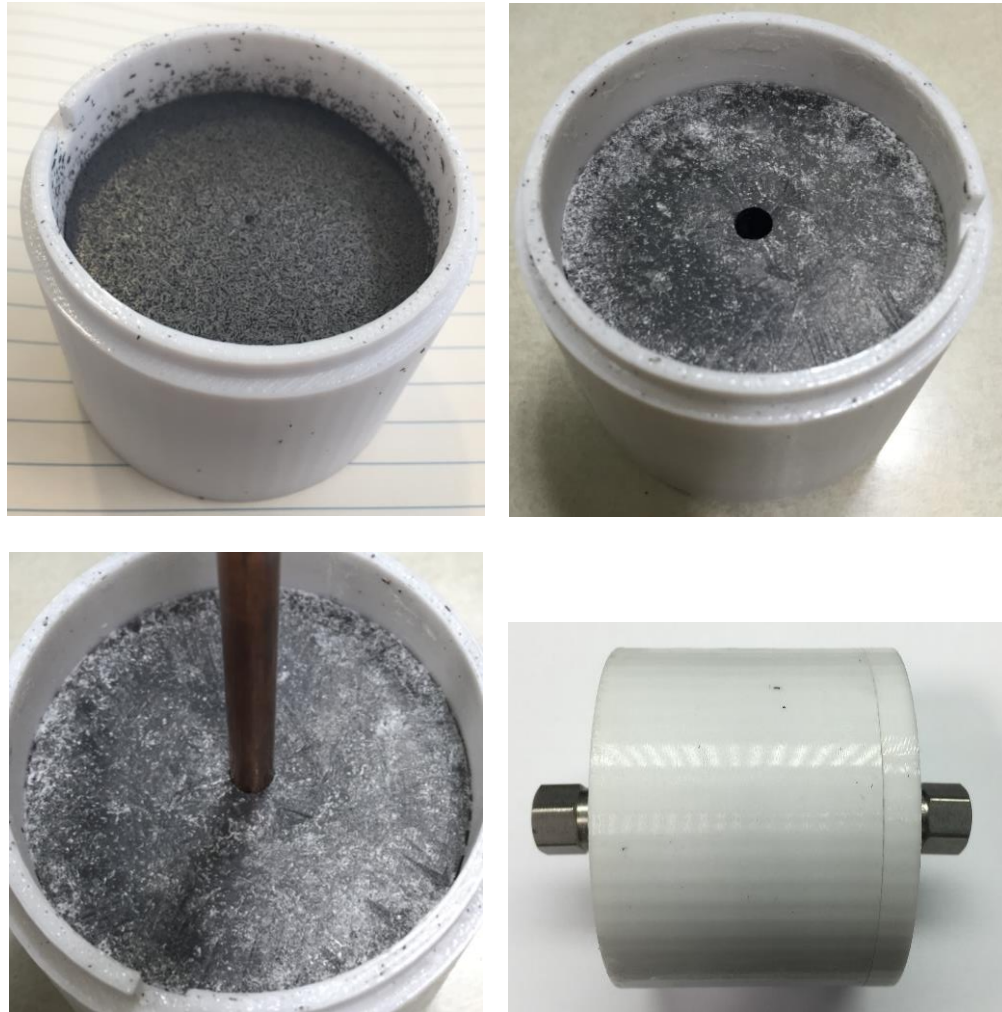
Figure 5.16. CENG within test container (top left); CENG following saturation and drilling of tube hole (top right); Installation of copper tube (bottom left); Final product (bottom right).
